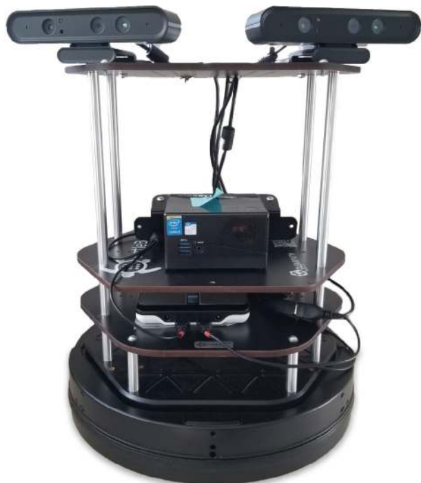
FIGURE 22. Turtlebot2 with camera setup.
