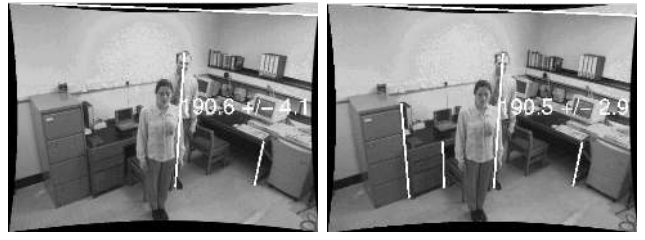
Figure 9: Uncertainty analysis on height measurements: The image shown was captured from a cheap security type camera which exhibited radial distortion. This has been corrected and the height of the man estimated (measurements are in cm). (left) The height of the man and the associated uncertainty are computed as 190.6cm ( c.f. ground truth value 190cm). The vanishing line for the ground plane is shown in white at the top of the image. When one reference height is used the uncertainty (3-sigma) is \pm 4.1 cm, while (right) it reduces to \pm 2.9 cm as two more reference heights are introduced (the filing cabinet and the table on the left).
