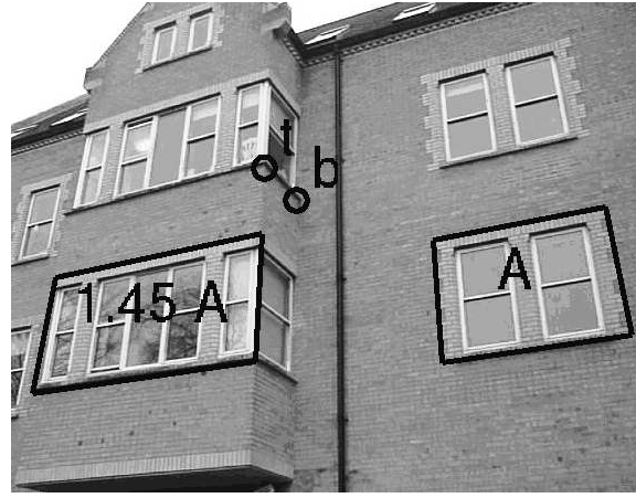
Figure 7: Measuring ratios of areas on separate planes: The image points t and b together with the vanishing line of the two parallel planes and the vanishing point for the orthogonal direction define the homology between the planes. The ratio between the area of the window on the left plane and that of the window on the right plane is computed.
