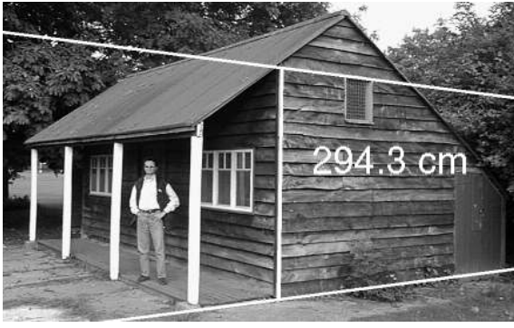
Figure 6: Measuring heights using parallel lines: Given the vertical vanishing point, the vanishing line for the ground plane and a reference height, the distance of the top of the window on the right wall from the ground plane is measured from the distance between the two horizontal lines shown, one defined by the top edge of the window, and the other on the ground plane.
