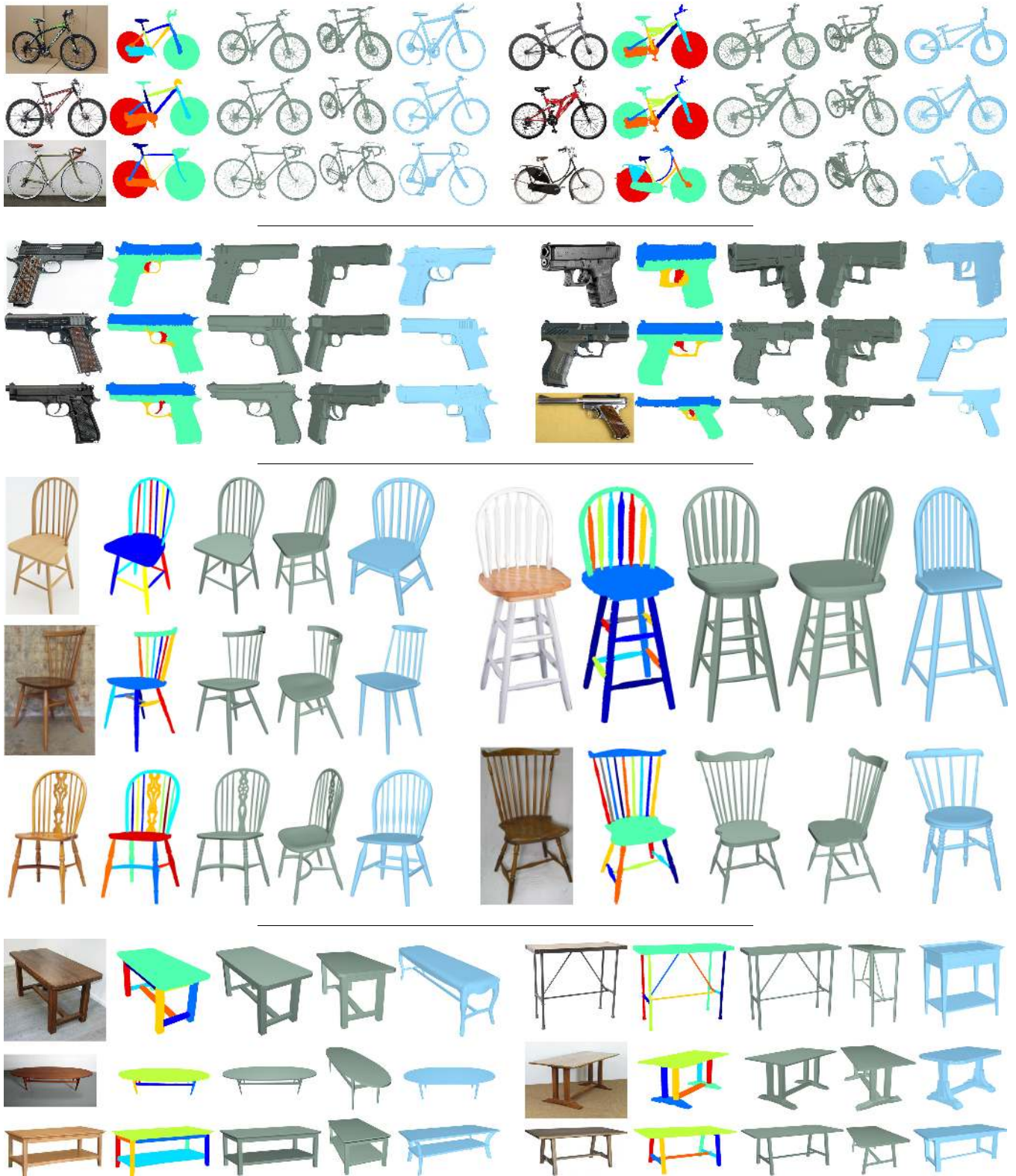
Figure 8: Results on four datasets. From left to right in each column: Web image, computed segmentation, 3D model reconstructed by our approach (two views, green), and closest pre-existing model, shown for reference (blue).
