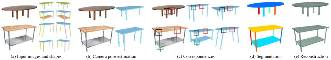
Figure 2: Stages of the presented approach. (a) Input: natural images and pre-existing 3D models. (b) Camera pose estimation for natural images, visualized by showing pre-existing models from the estimated poses. (c) Correspondence structure via a dense network of patches that interconnect natural images and rendered images. (d) Joint image segmentation. (e) 3D reconstruction of each natural image using parts from pre-existing models.
