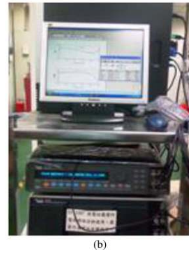
Fig. 6. Pictures of (a) the battery-charging test platform and (b) the ac-impedance analyzer.
