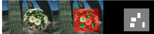
Figure 2. The original image from [11], a user provided rectangular selection (red: region of interest, green: known foreground), and the corresponding trimap (black: known background, gray: unknown, white: known foreground).
