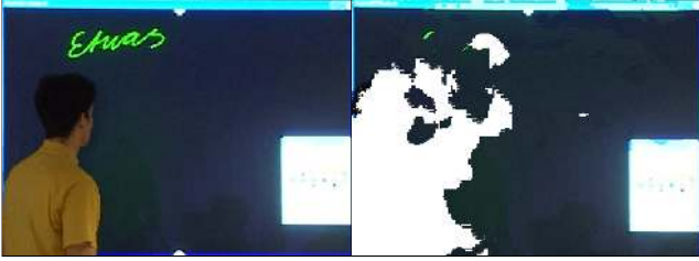
Figure 9. For extracting foreground objects in a video the trimap has to be reconstructed from motion statistics. The images show the original video (left) and known background that was reconstructed over several frames (right). The white regions constitute the unknown region.
