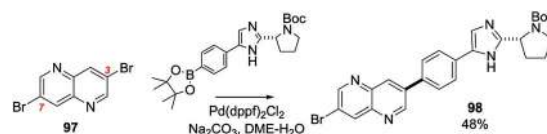
Scheme 27 A SMC reaction of 3,7-dibromo-5-azaquinoline with pinacolborane ( 97 → 98 ). 69
