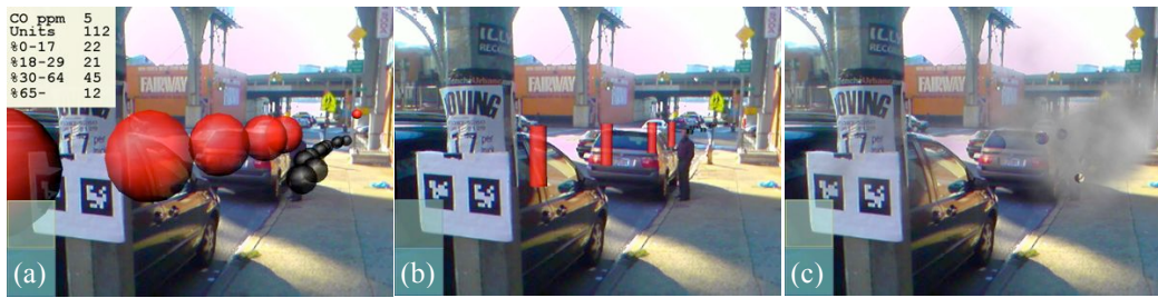
Figure 1. (a) Combining a screen-fixed readout (upper-left) with world-fixed data representation using spheres. Two alternative representations of the same data: (b) cylinders, and (c) smoke.
