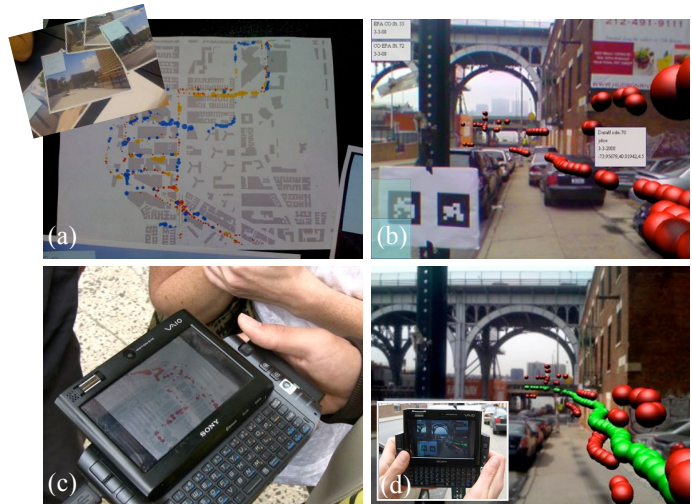
Figure 1. (a) Map of CO sensor data and photographs to provide context for the sensor data. (b) First iteration of SiteLens with data panels (gray boxes in upper-left corner) and detail pane (gray box in middle-right). (c) Dynamic map view. (d) Comparing locally sensed data (red) and remote EPA sensor reading associated with the site (green).
