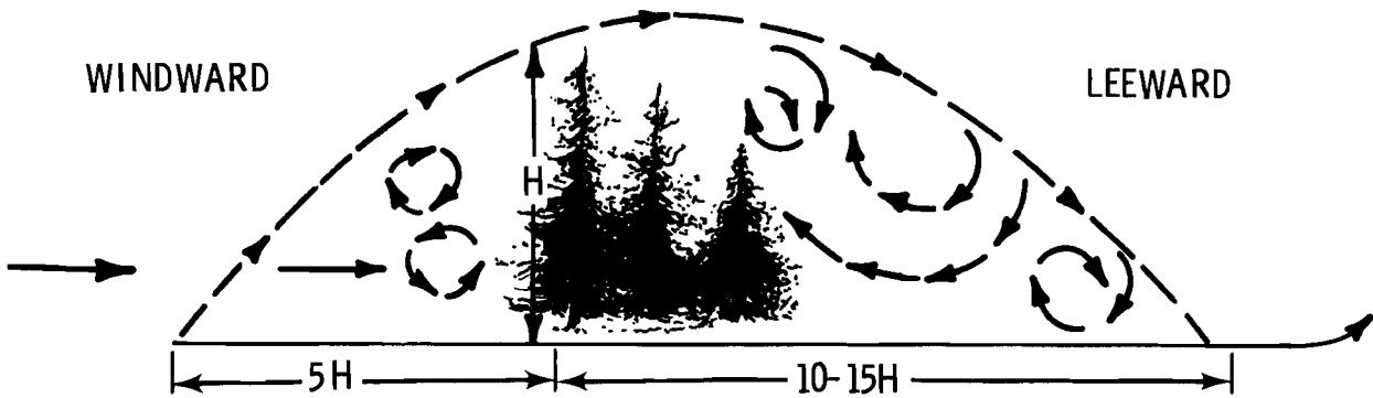
FIGURE 13. Airflow Near a Shelterbelt (Van Eimern et al., 1964)
