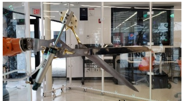
Scissor end-effector mounted to robot and actuated
