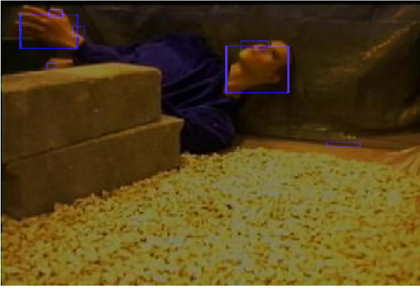
Fig. 5. Victim recognition. Skin textures particles obtained by on-line re-sampling for mixture models, are clustered and a skin region is highlighted. Picture from the Lisbon red arena
