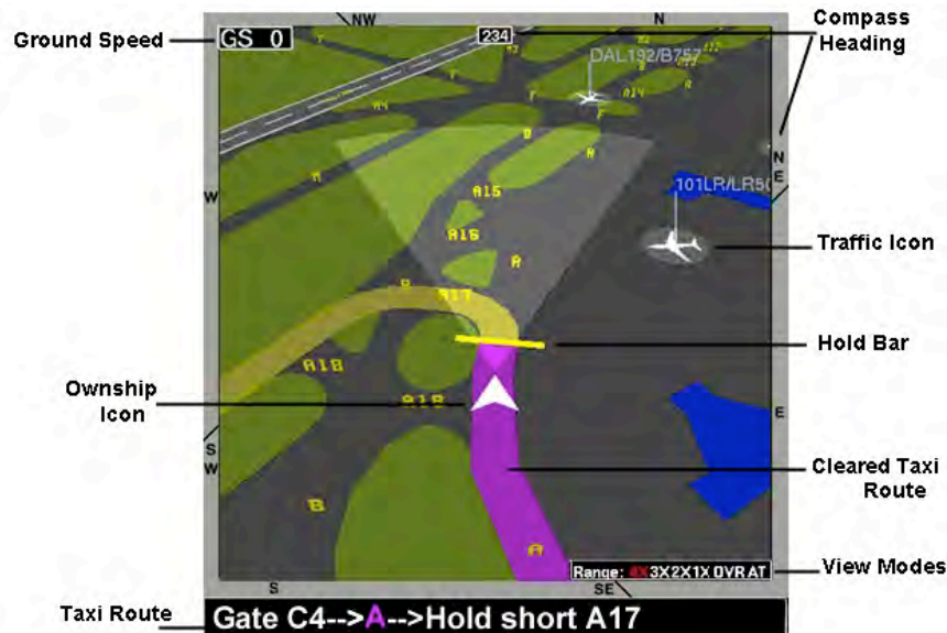
Figure 4. T-NASA panel-mounted, exocentric perspective EMM, with display elements labeled. Shown is the ownship aircraft taxiing at Chicago's O'Hare airport; the ownship is holding for another aircraft, with planned route curving to the left. The "wedge" is the large, triangular highlighted area with apex at the top of the ownship icon.
