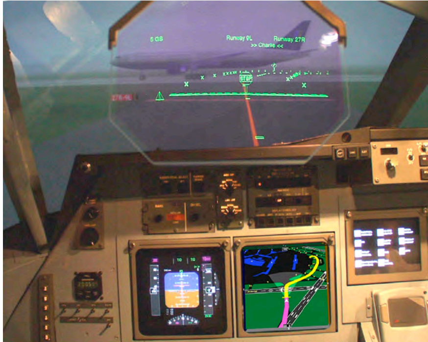
Figure 2. The T-NASA (Taxiway Navigation and Situation Awareness) system is composed of a transparent head-up display (HUD) using augmented-reality scene-linked symbology (top); and a panel-mounted electronic moving map (EMM, bottom middle-right).
