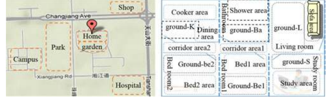
Fig. 6. Fine-grained radio map for outdoor (left) and indoor (right) environments.
