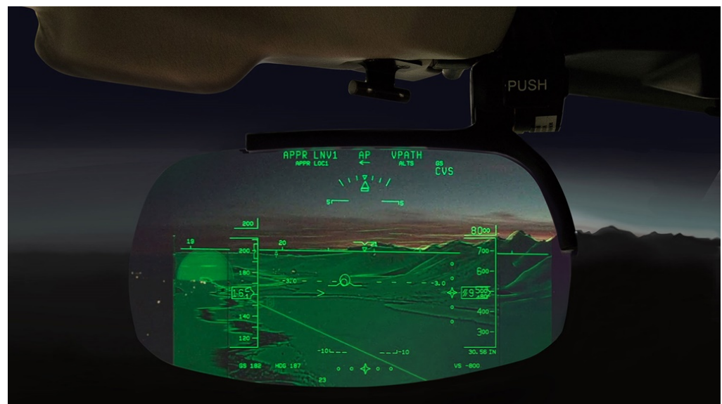
Figure 4. Collins Aerospace's Combined Vision System [43].
