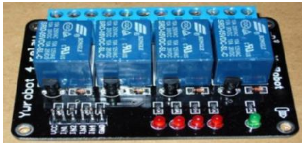
Figure 6. Relays board with their driver
