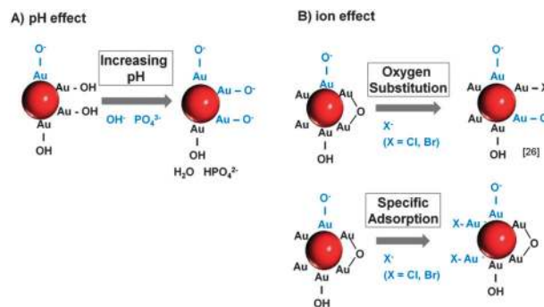
Fig. 11 Mechanisms of surface charge generation on ligand-free Au NPs by (A) pH changes and (B) specific ion effects.
