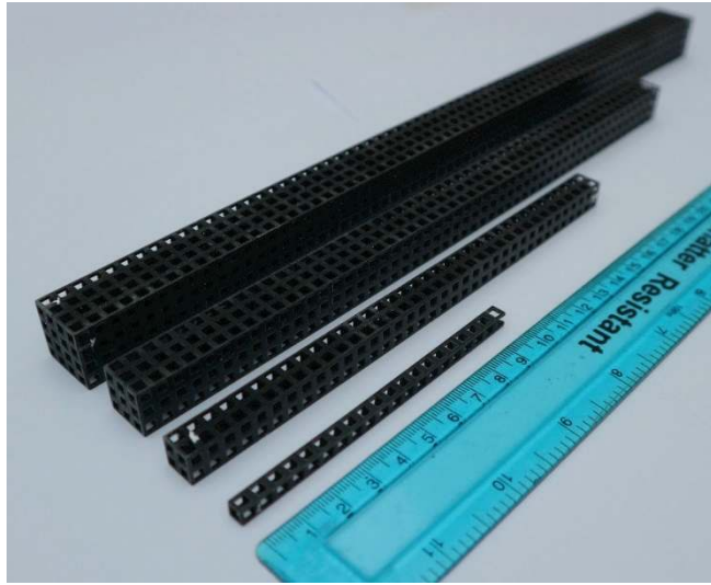
Figure 1: Metamaterial samples of various sizes for flexural testing
