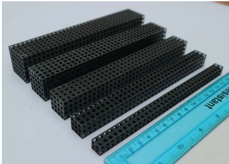
Figure 2: Metamaterial samples of various sizes for torsion testing
