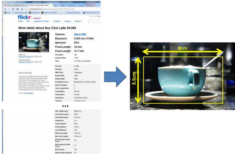
Figure 2: Illustration of metric object size derived from image metadata stored in EXIF fields on an image downloaded from Flickr.com. Absolute size is estimated by projecting bounding box of local features on object into 3-D using EXIF camera intrinsics stored in image file format.
