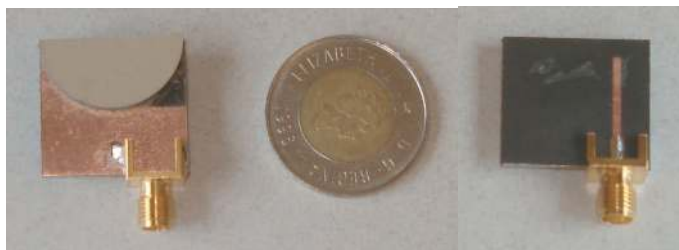
Figure 1. Geometry of the proposed UWB antenna. (a) Antenna configuration. (b) Photo of the optimized antenna prototype.
