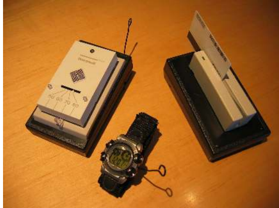
Figure 5. ECC-enabled wireless devices built at Sun Labs: (a) thermostat, (b) health-monitoring watch (c) magnetic stripe reader.
