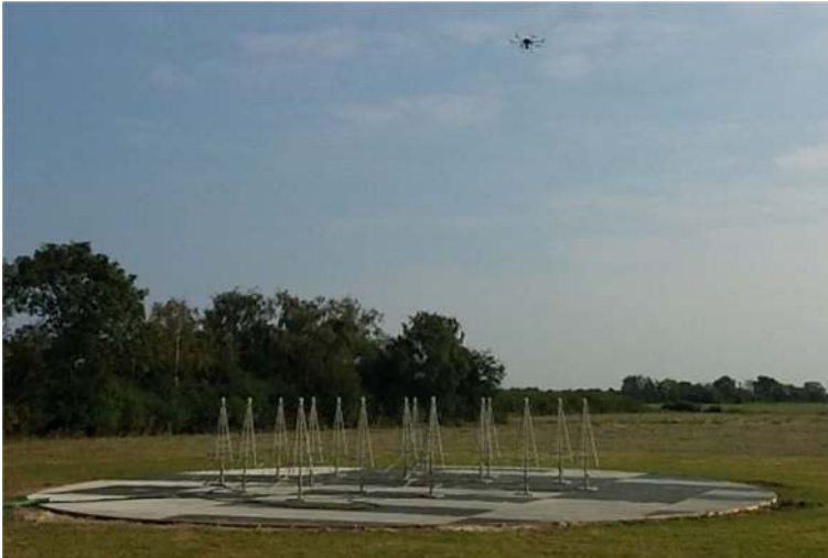
Fig. 3 UAV flying over the AAVS0 array, deployed at the Mullard Radio Astronomy Observatory, Lords Bridge, Cambridge
