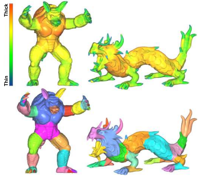
Figure 10: (Top) A visualization of the local thickness at each skeleton node. (Bottom) Segmentation results.
