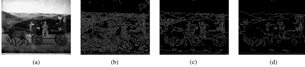
Fig. 1. Effect of \beta parameter on edge maps. (a) Model image, (b) \beta = 1 , (c) \beta = 2 , (d) \beta = 3 .
