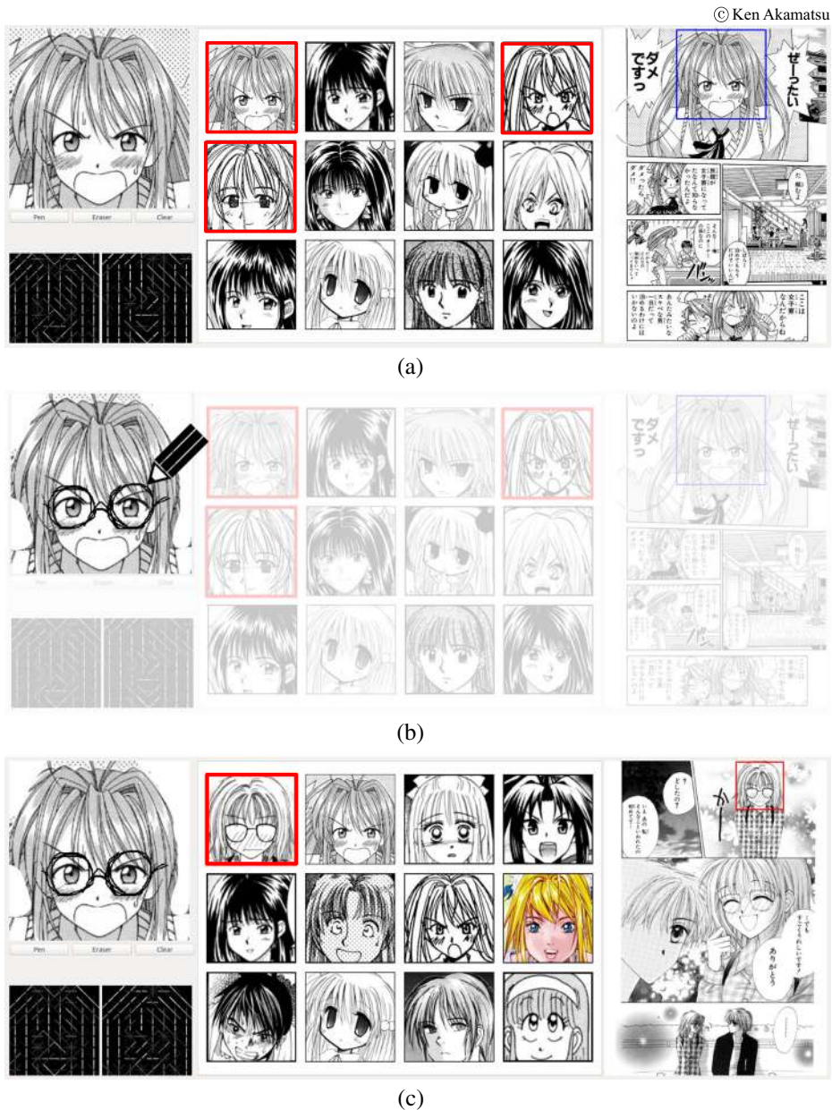
Fig. 10 Query retouch. a Results of relevance feedback. Target characters have red borders. b A user adds strokes and draws glasses on the target character. Other target characters with glasses are then successfully retrieved (red borders). Note that users can erase lines using an eraser tool. c Both relevance feedback and query retouch can be conducted multiple times
