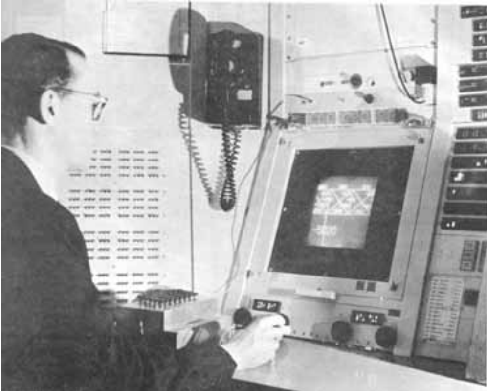
Figure 1.2: TX-2 OPERATING AREA — SKETCHPAD IN USE. On the display can be seen part of a bridge similar to that of Figure 9.6. The Author is holding the Light pen. The push buttons used to control specific drawing functions are on the box in front of the Author. Part of the bank of toggle switches can be seen behind the Author. The size and position of the part of the total picture seen on the display is obtained through the four black knobs just above the table. ( Originally on page 11. )
