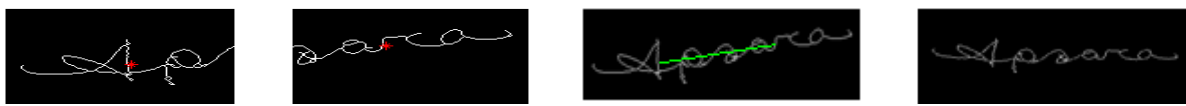
Fig. 13 Skew angle detection using center of gravity a) Center of gravity in left half b) Center of gravity in right half c) Join the two center of gravities d) Skew free signature
