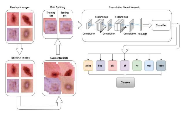
Figure 2. Overview of the proposed ESRGAN-based CNN algorithm.
