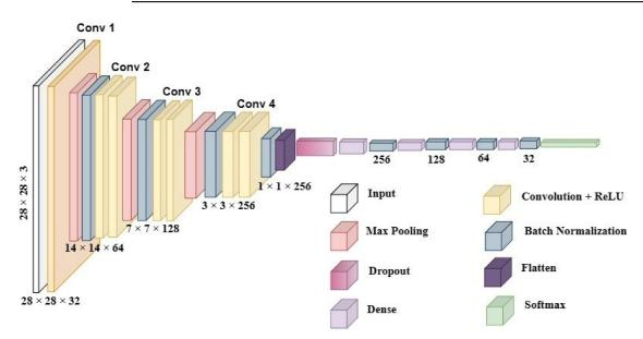
Figure 3. Layered architecture of proposed CNN model.
