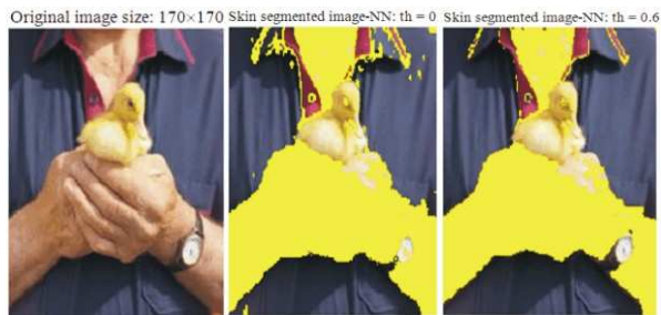
Fig.7: (From left to right) original image-3, segmented image-3 with \theta = 0 and segmented image-3 with optimum threshold \theta = 0.6
