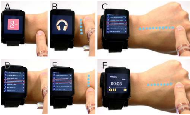
Figure 11. Swiping up or down navigates between apps (A,B). Swiping right launches the selected app (C). Sliding can also be used to continuously scroll a playlist (D,E); swiping right plays the selected song.
