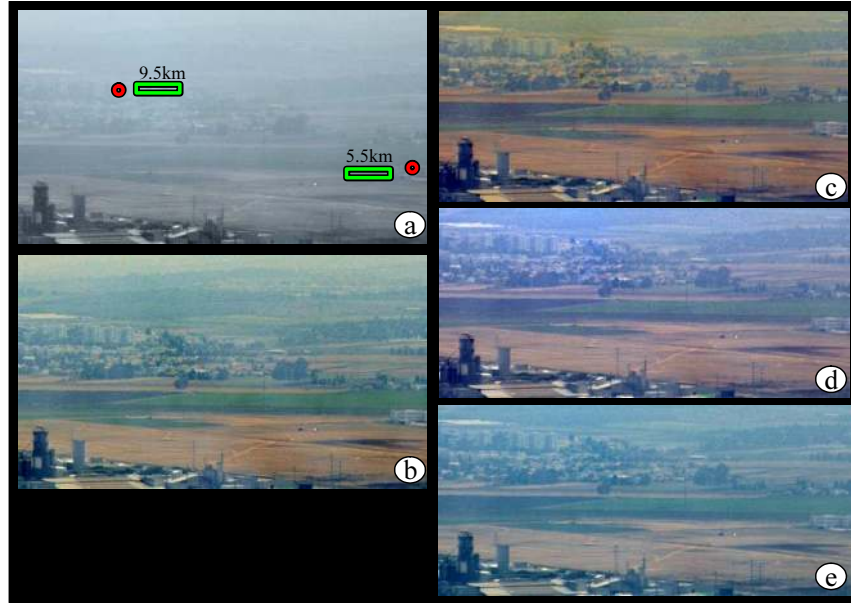
Fig. 9. Dehazing of Scene 3 , whose distances are up to 13.5 \text{ km} . The scene contains smoke. (a) The best polarized raw image. (b) Sky-based dehazing. (c) Result of a feature-based method assisted by ICA (d) Result of a distance-based method assisted by ICA (e) Distance-based result.
