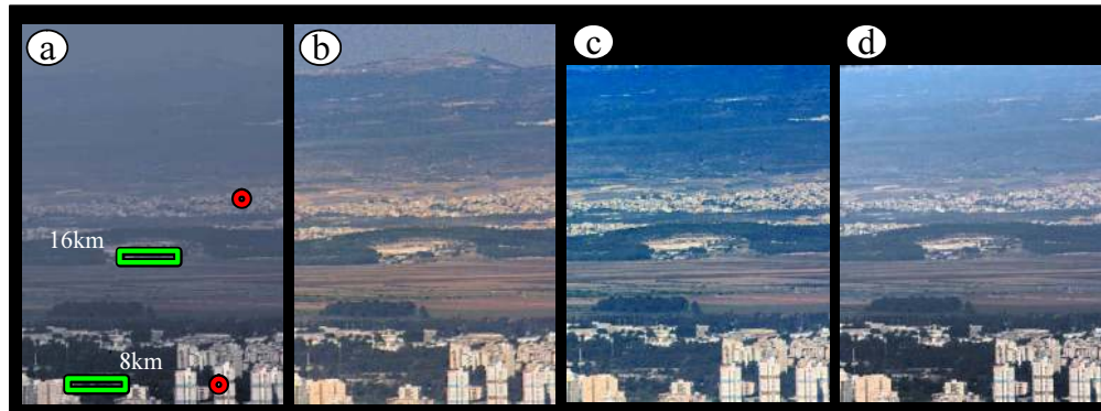
Fig. 10. Dehazing of Scene 4 , whose distances are up to 31 \text{ km} . (a) The best polarized image. (b) Sky-based dehazing. (c) Result of a feature-based method assisted by ICA (d) Result of a distance-based method assisted by ICA (e) Distance-based result.
