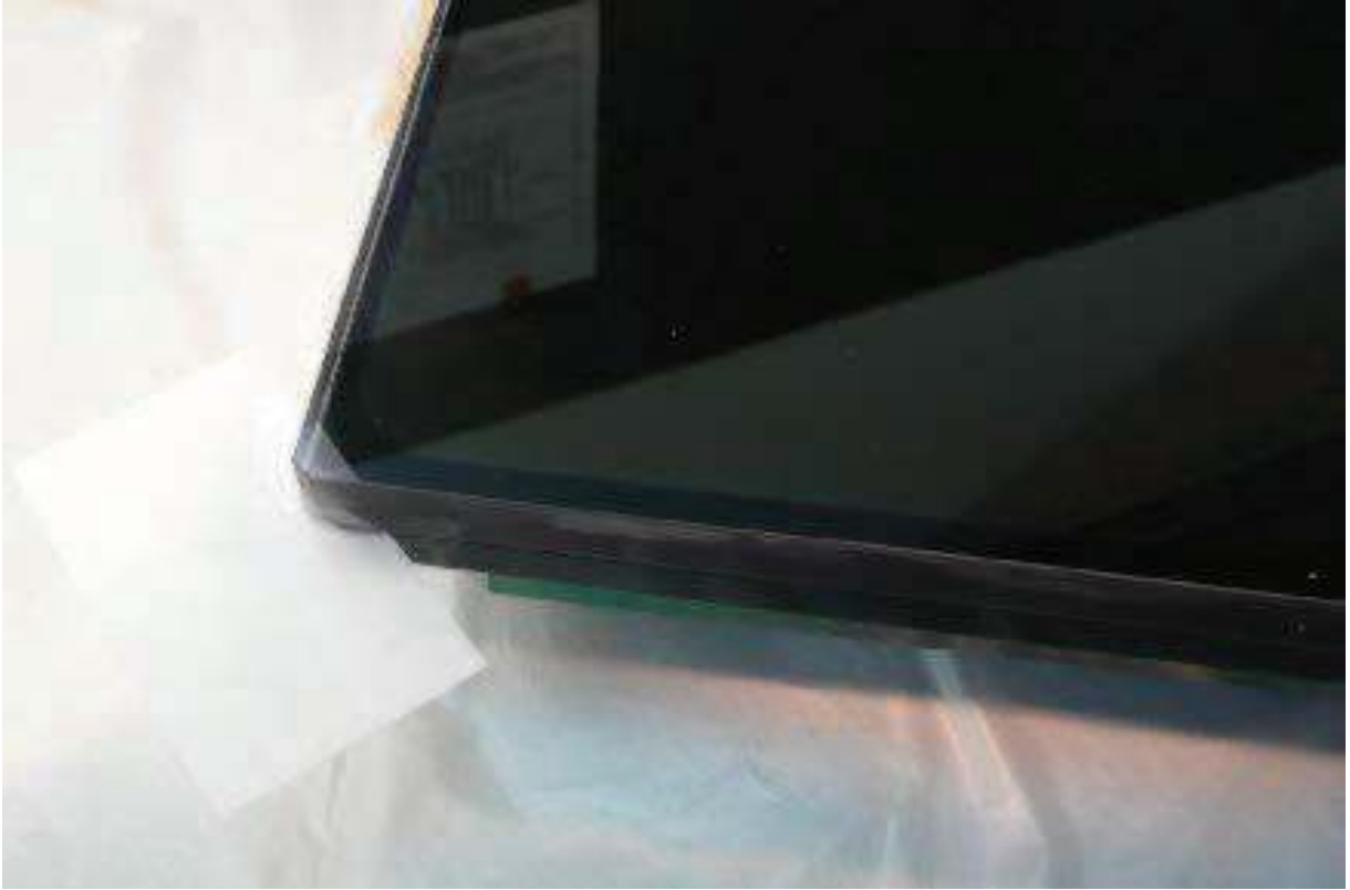
Fig. 2.— The last mylar shim in place while gluing the u filter
