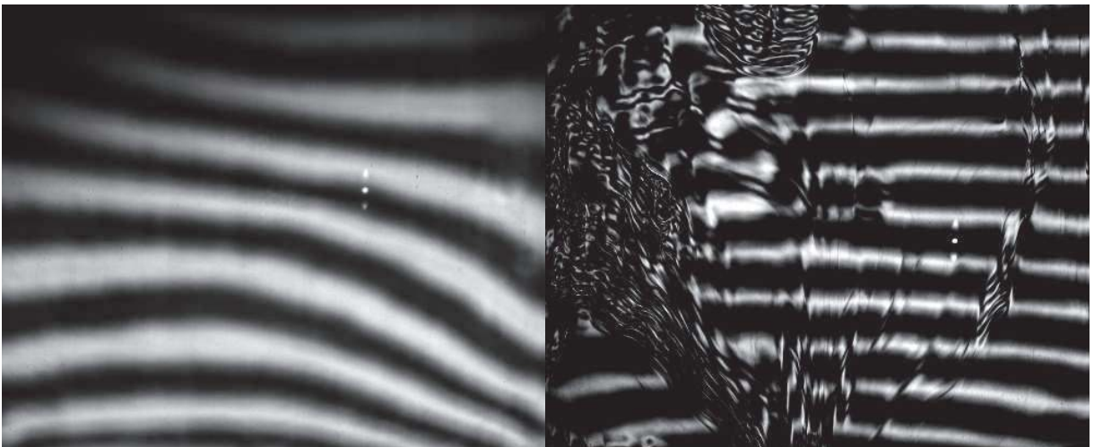
Fig. 3.— Ronchi fringes through good and bad sections of a rejected filter.
