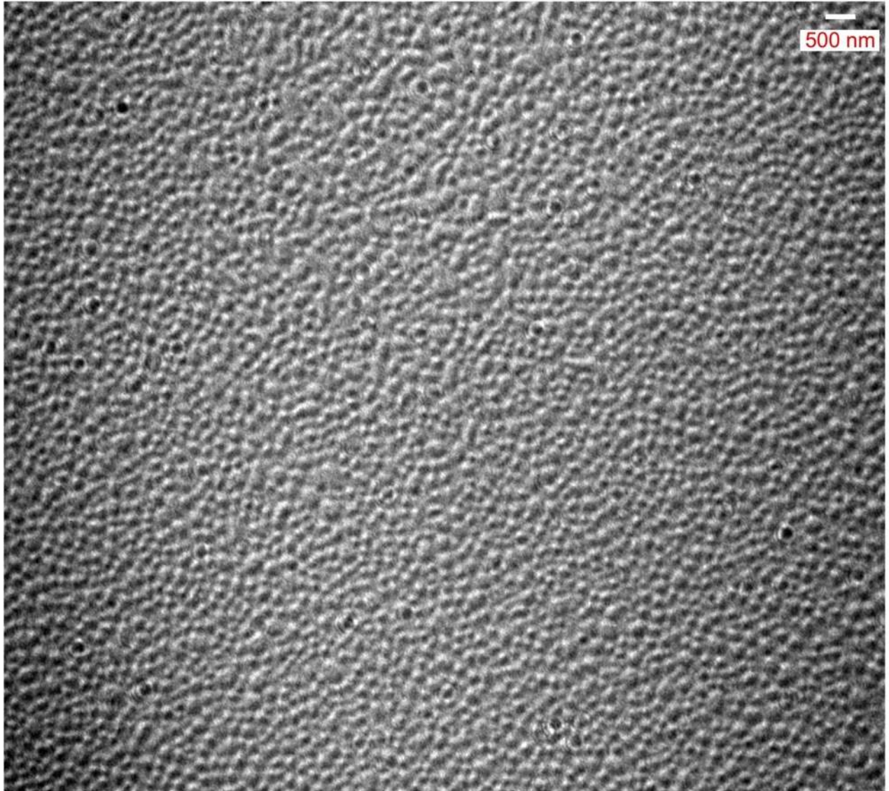
Fig. 25. Lorentz TEM imaging data acquired in a [\text{Pt}/\text{Co}/\text{Ir}]_8 multilayer. Note that these densely packed Néel-type skyrmions were stabilized at room temperature in the absence of magnetic fields. A multilayer of \text{Ta}(2\text{nm})/[\text{Pt}(1.5\text{nm})/\text{Co}(1\text{nm})/\text{Ir}(1\text{nm})]_8/\text{Pt}(1.5\text{nm}) was grown by using dc magnetron sputtering under a 3 mTorr Ar pressure onto 2 \times 2 \text{ mm}^2 TEM grids with 50 nm thick silicon nitride (SiN) membrane window. The zero-field Lorentz TEM experiments were performed in a JEOL 2100F instrument with a spherical aberration corrector. The corresponding out-of-focus Fresnel imaging mode was used with a defocus value of 6.4 mm. The sample was tilted 30 degree along the diagonal direction to gain magnetic contrast (manuscript in preparation by Wanjun Jiang, et al.).
