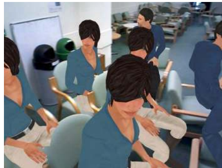
Figure 9. Context-aware augmented reality: virtual characters navigate the mapped scene and automatically find sitting places.
