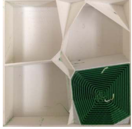
Figure 17: One of the interior cells filled with offsets.
