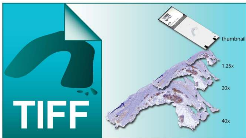
Figure 2. A visualisation of a multi-page pyramid TIFF file. This illustration shows a TIFF file with 4 layers (thumbnail, 1.25x, 20x, 40x), digital slides stored as TIFF files often contain up to 11 or more layers. doi:10.1371/journal.pone.01110289.g002
