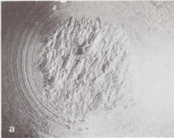
Slider Tested at 760 Torr X20
