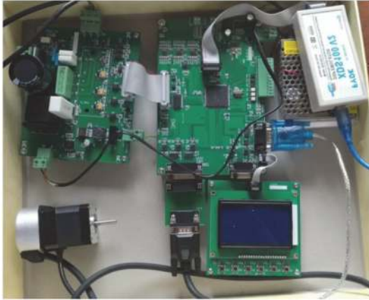
FIGURE 12: Experimental platform for the SPMSM control system.
