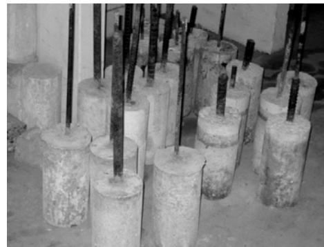
Figure 7: Samples ready for pullout test.
