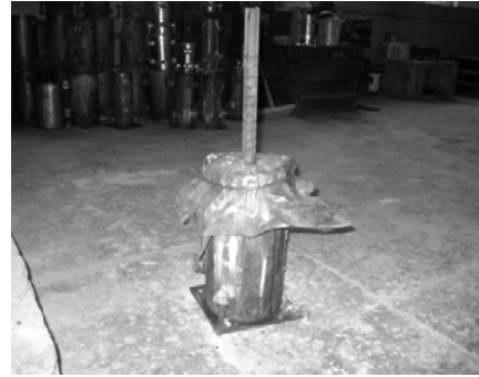
Figure 5: Pullout sample immediately after casting..
