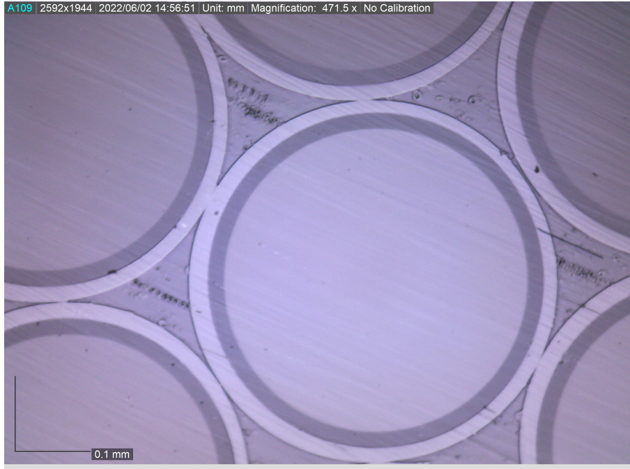
Figure 10: Typical end-finish after polishing object fibres in 400 \mu\text{m} diameter core fibre IFU.
