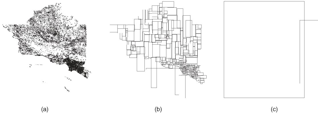
Fig. 7. Entries of T1 R*-tree. (a) Level 0 (leaf) entries. (b) Level 1 entries. (c) Level 2 (root) entries.
