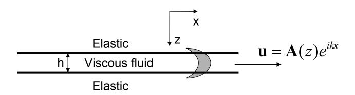
Figure 1. A layer filled with viscous fluid between two elastic halfspaces
