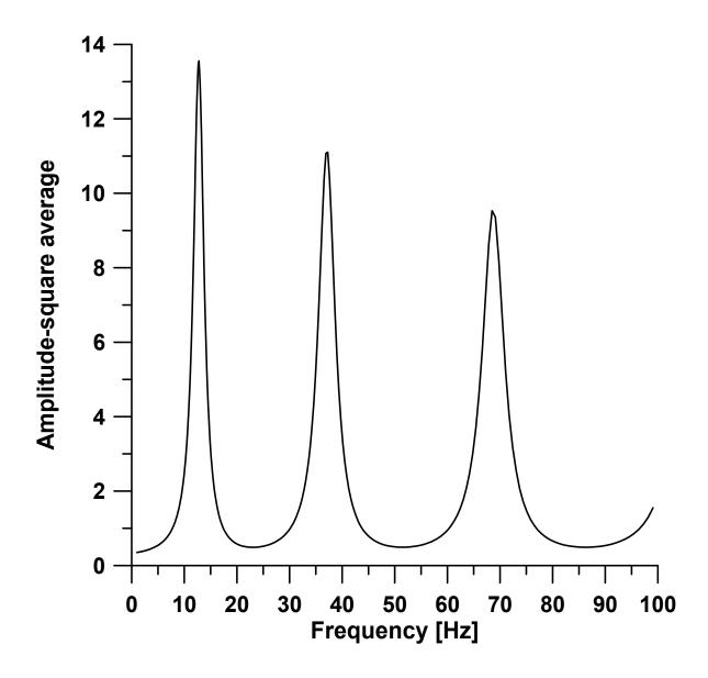
**Figure 5.** Resonant energy density for 4 m long 1 mm thick water-filled fracture.
