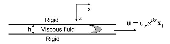
**Figure 2.** Biot's model for flow in fractures. Interaction of fluid with the fracture walls occurs because of the friction forces. Fluid motion goes predominantly along the rigid walls.
