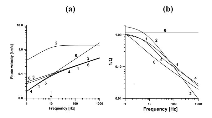
**Figure 4.** Same as in Figure 3, but for oil-filled fractures. The small *S* asymptotic provides a good approximation for the exact solution, which differs significantly from the nonviscous fluid solution. The values of Q at seismic frequencies reach 10.
