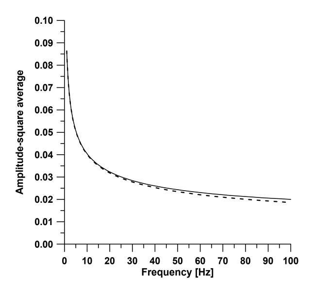
**Figure 7.** Amplitude-square average for a "thin" fracture filled with oil. Exact solution (solid line) is compared with analytical approximation given by equation 51 (dashed line). Low frequencies yeald higher amplitude responses.
