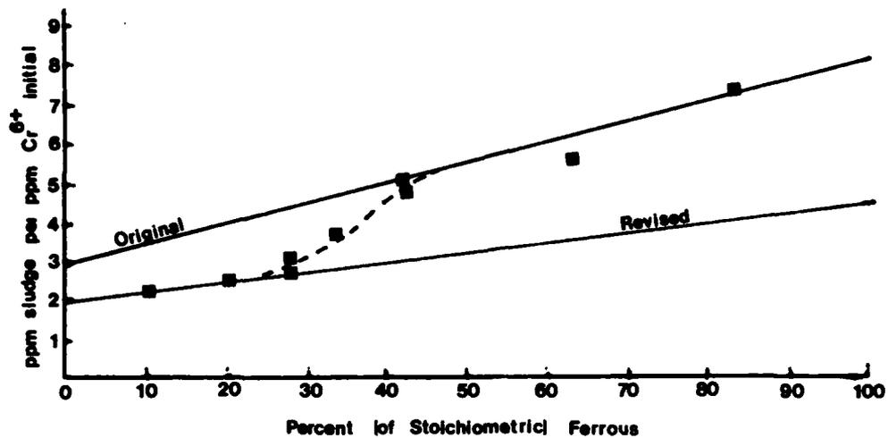
Figure 10. Catalytic Effects of Iron on Sludge Production
