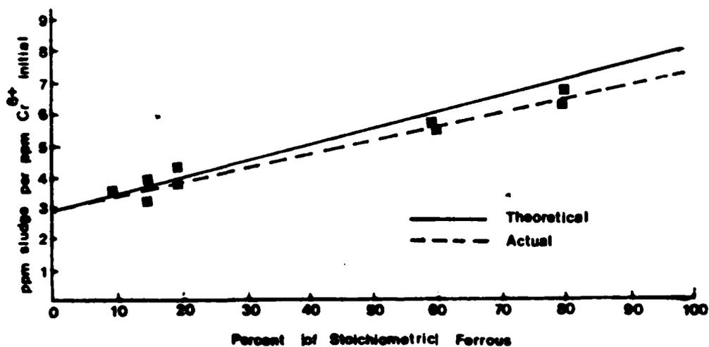
Figure 6. Sludge Production from Alkaline (pH 10.0) Chromium Reduction.
