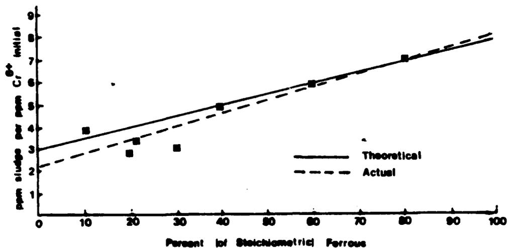
Figure 5. Sludge Production from Alkaline (pH 8.0) Chromium Reduction.
