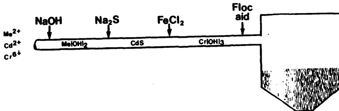
Figure 11. One Step Treatment Schematic
