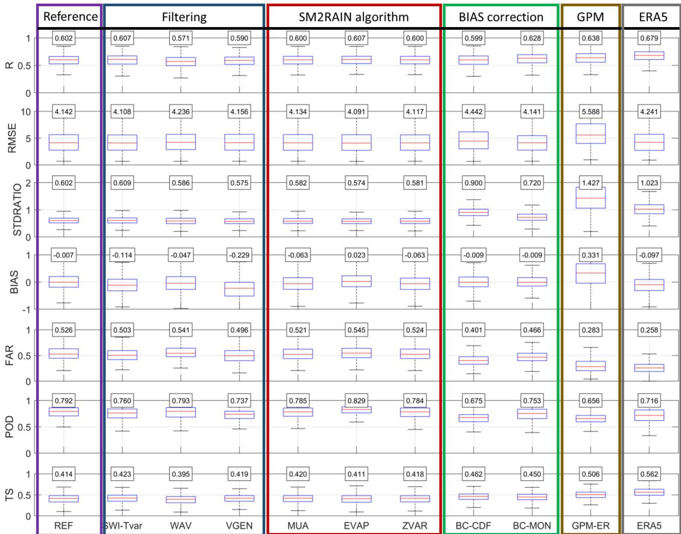
Figure 3. Performance at 1009 points in terms of Pearson's correlation, R (–), root mean square error, RMSE ( \text{mm d}^{-1} ), the variability ratio, STDRATIO (–), the mean error between estimated and reference rainfall, BIAS ( \text{mm d}^{-1} ), the false alarm ratio, FAR (–), the probability of detection, POD (–), and the threat score, TS (–). For details about the different configurations see Table 2 (GPM-ER: GPM IMERG Early Run product).
