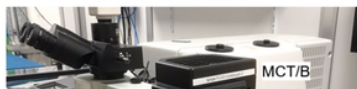
(a) Near- and Mid-IR setup : Continuum microscope, FTIR spectrometer (Thermo Fisher) with MCT/B detector
