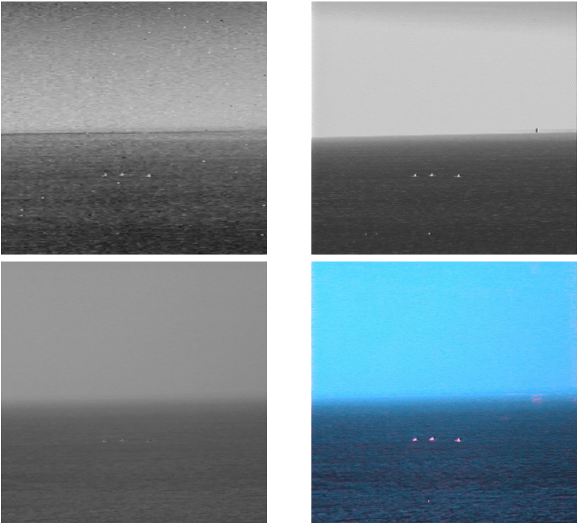
Fig.4. Upper row: corresponding original Radiance 3-5 \mu\text{m} (left) and AIM 8-12 \mu\text{m} (right) IR images. Lower row: corresponding original CCD (left) and fused (right) images.
