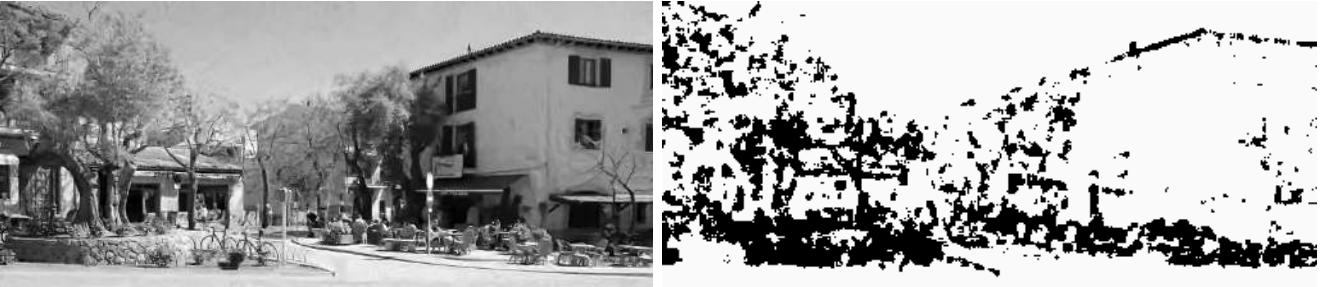
Figure 4: SSaNN forms a new image (left) by replacing texture pixels in BM3D’s restored image with those estimated by the neural network. Pixels identified as part of the texture are marked in black in the right image. This combination enables a RMSE reduction from 12.34 to 12.15.
