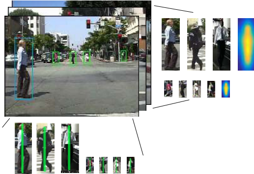
Fig. 1. Pedestrians over different scales could be modeled as a group of 2D Gaussian kernels, indicating that the top-bottom topological line possess high certainty. Our approach attempt to locate this topological line for pedestrian detection.
