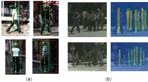
Fig. 7. (a) Samples of our detection results (green) and GT boxes (red) in KITTI validation set. (b) The effectiveness of our predicted link map in crowd scenes.
