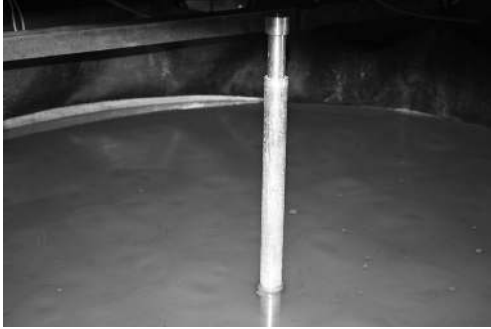
Figure 3: The 40 mm pile installed in the sand in the pressure tank.
