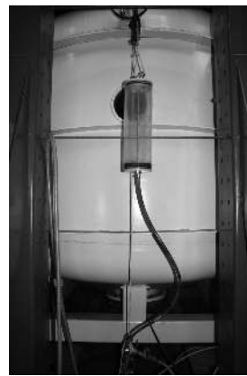
Figure 9: The ascension pipe connected to the tank to maintain hydrostatic pore pressure in the soil during the tests.
