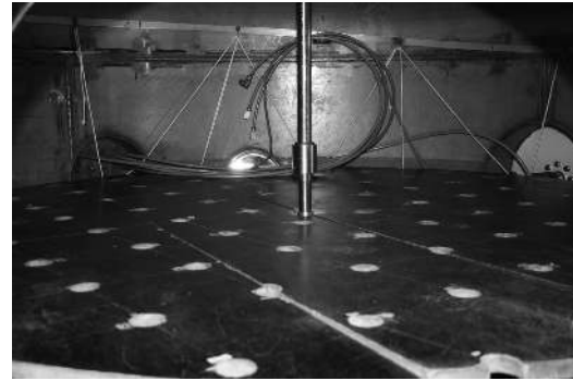
Figure 11: The pile fixed by the hydraulic piston.
