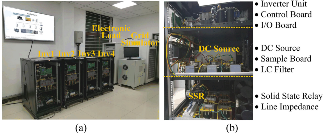
Fig. 28. Hardware platform of parallel inverters: (a) overall view and (b) inside view of each inverter.
