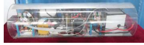
FIGURE 8: Physical picture of marine electromagnetic transmitter circuit.
