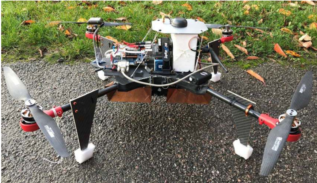
Fig. 2. Photograph of the small drone with SAR measurement hardware.
